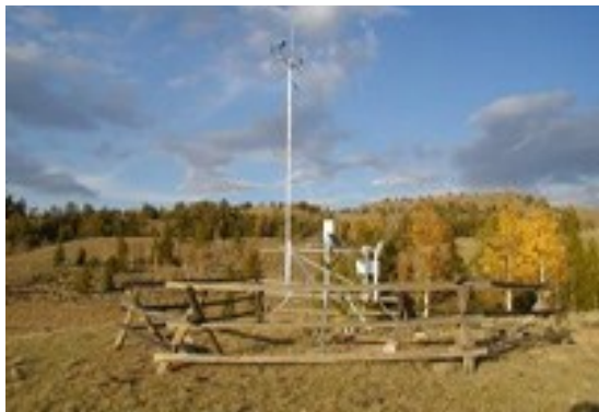
Above: A Forest Service Remote Automatic Weather Station
